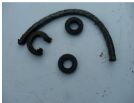
Graphite gland packing with the two Hydraulic seals
