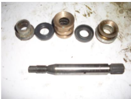
Above show the lead bushing, hydraulic seal, spacer, seal, brass
