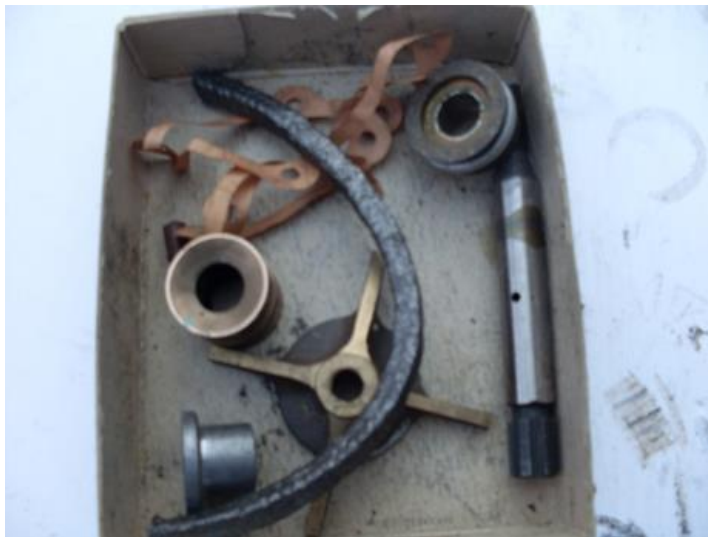
Water pump overhaul kit that includes paper gasket, shaft, impeller, lead and brass bushing,
