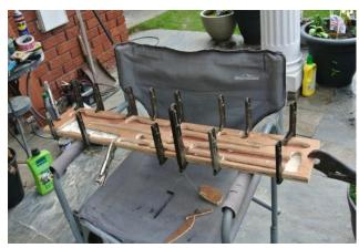
The last check, make sure the tools fit into the slots. This is important because once the felt is applied, you can not alter anything.
