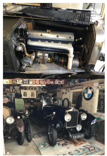
Bonnet open revealing the mighty six-cylinder Delage engine.
