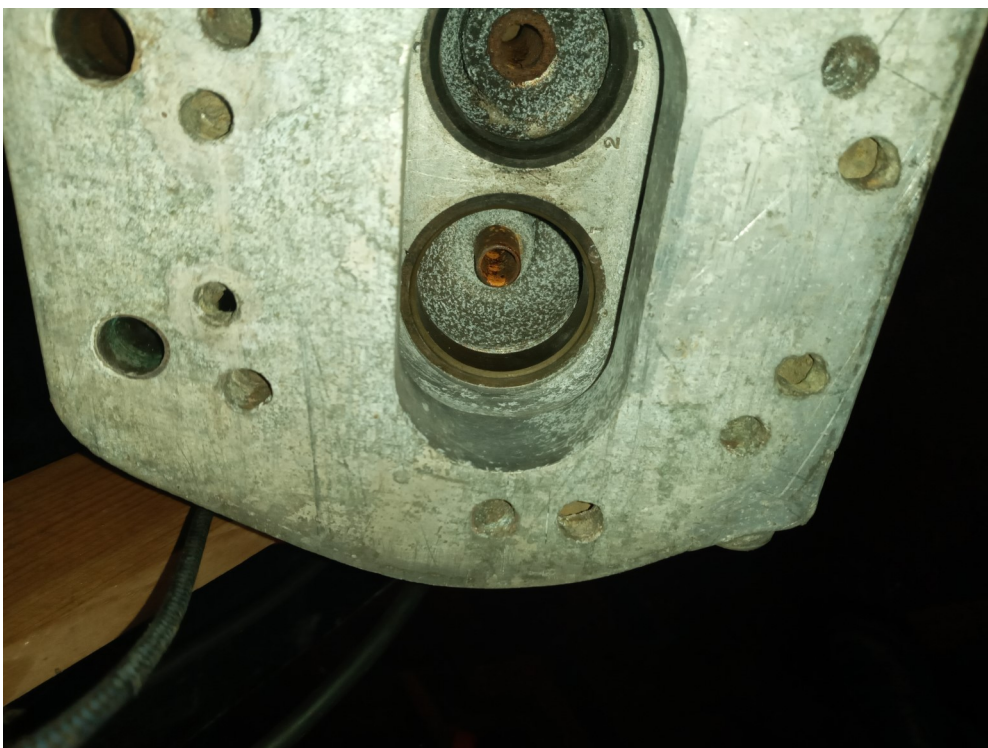
Left: Showing the valve seats in the aluminium head.
